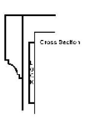
Molding nailed at corners, with 1/2" wooden dowels along sides and ends.
